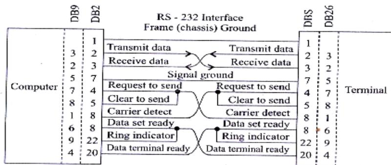
**: RS232 interface signal connections between computer and terminal device**
