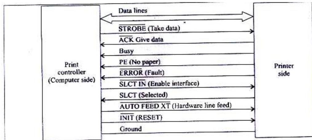
The Centronics Interface is a handshake protocol between a computer and a printer. It supports maximum data transfer speed of 100Kb/s. There are 12 signals from printer to PC. Out of these, 8 signals are data bits and four signals are control signals. All control signals are active low. The control signals are:
