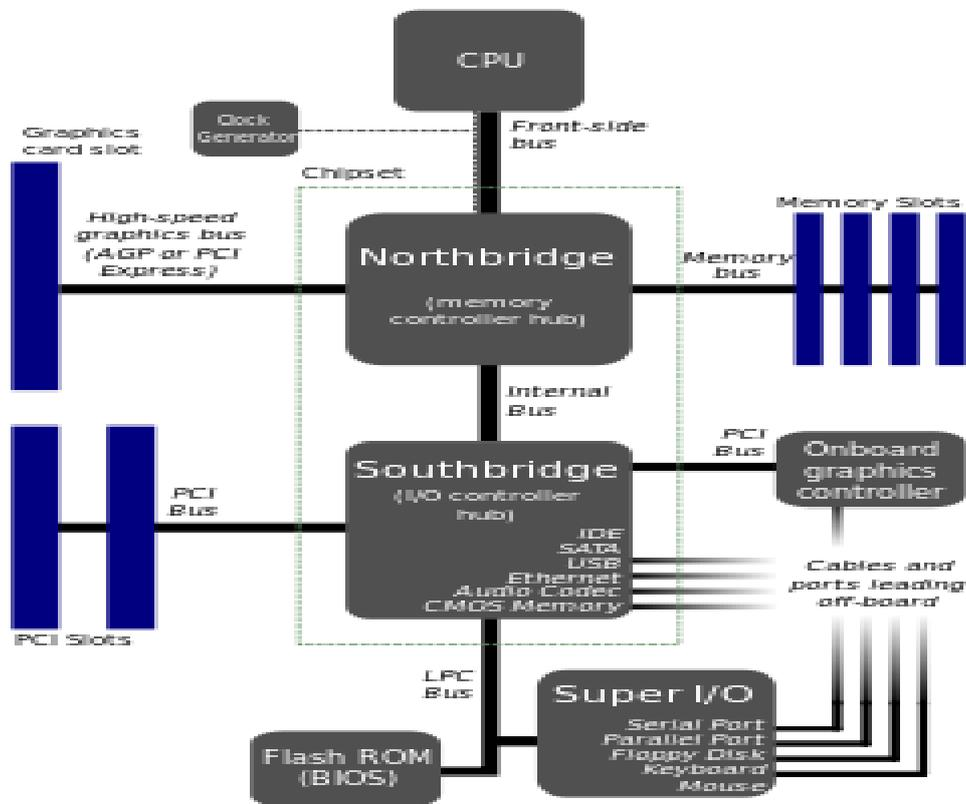
Intel's earlier chipset were broken into multi-tiered architecture known as North Bridge and South Bridge components as well as Super I/O chip. North Bridge: it is the connection between the high speed processor bus and the slower AGP & PCI buses. South Bridge: it is the bridge between PCI bus and even slower ISA bus. Super I/O chip: contains commonly used peripheral items all combined in single chip.
