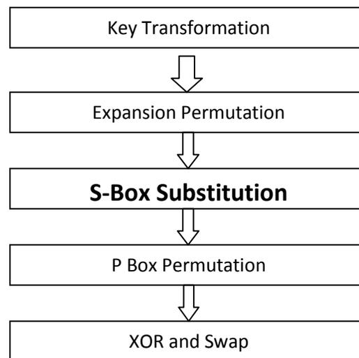
**Fig. Details of one round in DES**
