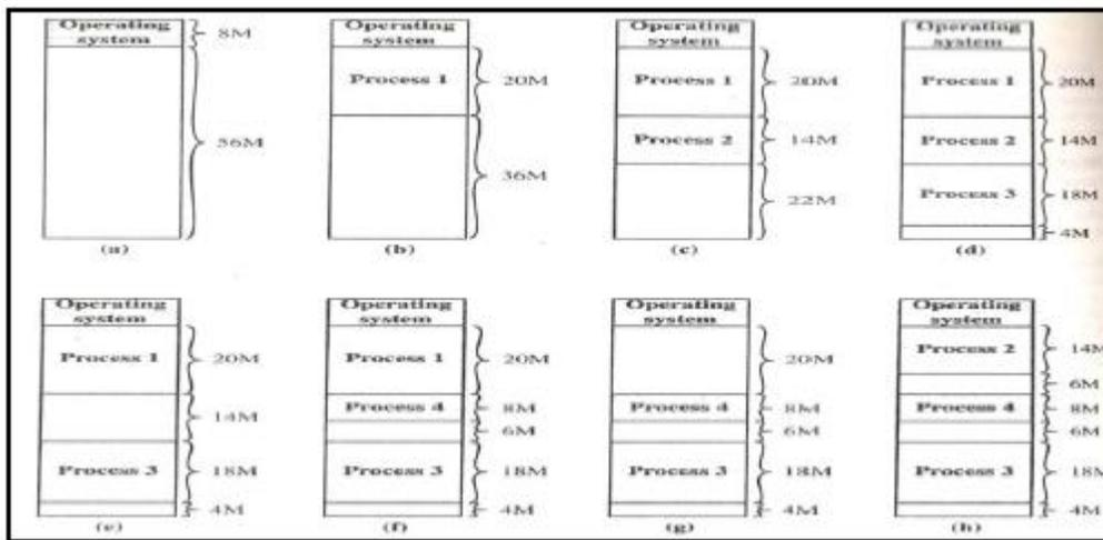
Total memory size is 64 M .From this 8 M partition is occupied by operating system and remaining can be partitioned as per the size of processes.
